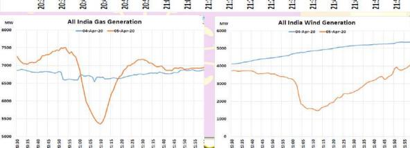
Reduction of total 10950 MW generation was achieved through Thermal (6992 MW), Gas (1951 MW) and Wind generation (2007 MW) during 20:45 Hrs to 21:10 Hrs.
