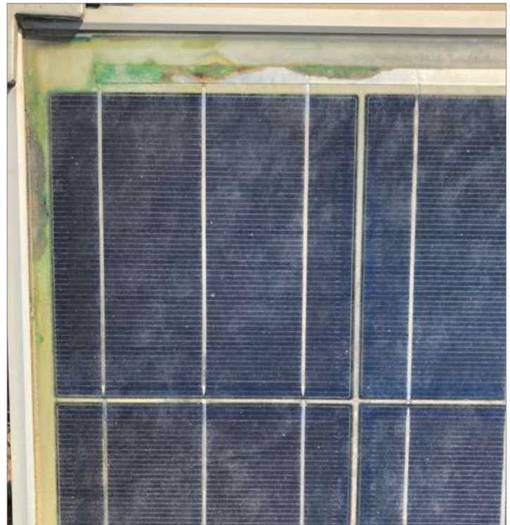
Damaged PV module from the field with evidence of busbar corrosion and delamination.
