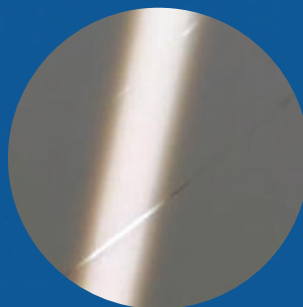
Widespread backsheet cracking PVDF
