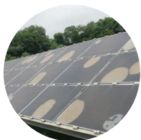
Glass/encapsulant delamination 8 years West India
