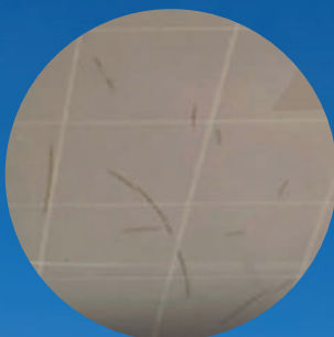
Widespread backsheet cracking PVDF
