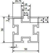
• Cross section Length: 50 process section Width: 50mm, Thickness: 02 mm
