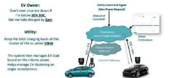
Figure 16: Illustration of basic requirements for managing EV clustering
