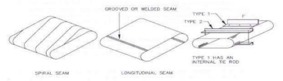
JOINTS AND CONNECTIONS ARE SIMILAR TO ROUND DUCT SIZE REINFORCEMENTS AS FOR RECTANGULAR DUCT OF F DIMENSION ATTACH REINFORCEMENT TO DUCT AT ENDS AND 12" (305 MM) MAX. SPACING
