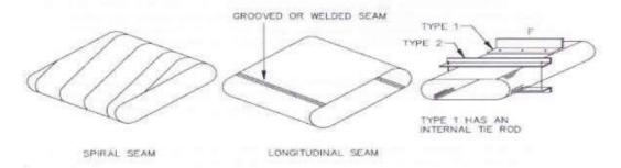
JOINTS AND CONNECTIONS ARE SIMILAR TO ROUND DUCT SIZE REINFORCEMENTS AS FOR RECTANGULAR DUCT OF F DIMENSION ATTACH REINFORCEMENT TO DUCT AT ENDS AND 12" (305 MM) MAX. SPACING
