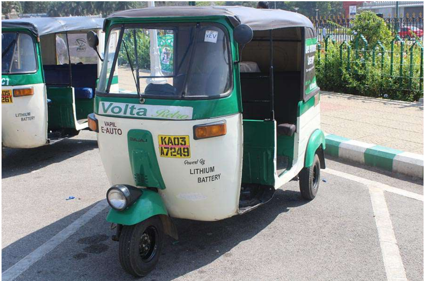
Figure 4: Retrofitted e-autorickshaw in India
