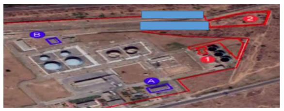
The area numbered 2 having Blue rectangle is selected for setting up the Solar PV Plant at HPCL Bihta Patna New IRD. The area is undulated and land grading levelling will have to be carried out.
