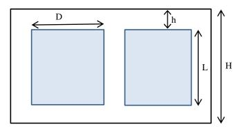
Net core area (A) =  $4056.52 \text{ cm}^2$ Window height (L) = 2000 mmYoke height (h) =740 mmCore Height (H) = L+ 2 x h=  $2000 + (2 \times 740) = 3480 \text{ mm}$ Window width (D) =810 mmLimb Pitch = D+h = 810+740 = 1550 mm
