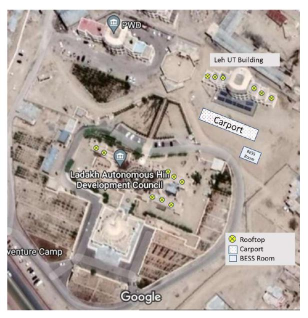
Note: The identified locations are tentative for installation of solar carport and rooftop systems, the actual area may be increased/decreased based on site assessments. As informed earlier, the area for solar shall be combination of rooftop and ground-mounted and land shall be made available with mutual discussions involving developer/client/CESL.
