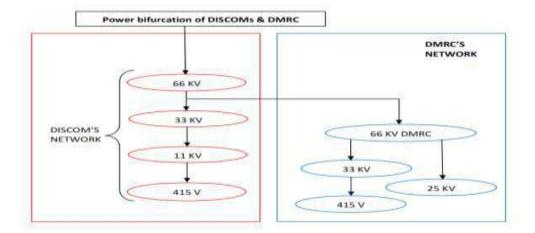
The above diagram shows very clearly that DMRC network is separated from the network of DISCOMs at 66 kV itself, hence it does not contribute in the losses of DISCOMs.
