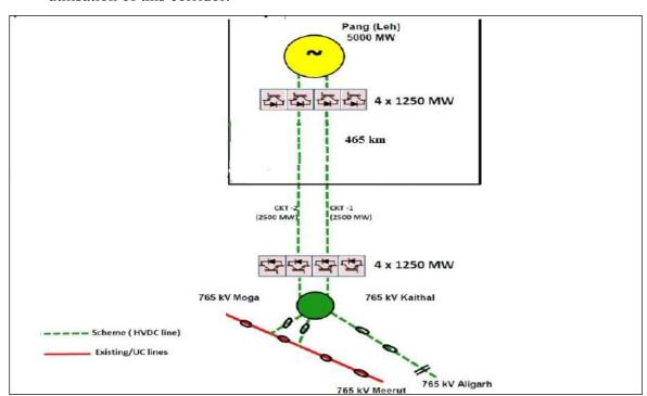
After deliberations in the 4<sup>th</sup> meeting of NRPC(TP), Pang- Kaithal VSC based HVDC system (5 GW) was agreed. Further, due to constraints observed in integration of the system with Moga and Aligarh, it was decided that the AC interconnections from VSC terminal at Kaithal would be worked out again and accordingly, intimated to constituents in the next NRPC(TP) meeting.
