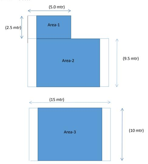
Total Approx. Available Area for Solar PV Array(with approx. 1.5- 3 meter extensions on either side ,over cantilever support erected on the Steel Structural Support as shown for the un-shaded area, shaded area has structural Concrete beams below). Additional area available on the roof-top can be utilized if required to meet the minimum requirement of 30KWp PV Panels.
