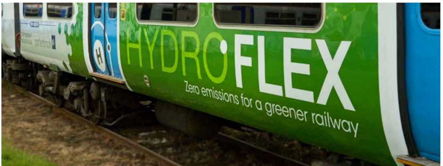
The 30-year-old Diesel Multiple Unit HydroFLEX vehicle has been converted to Hydrogen fuel cell power
