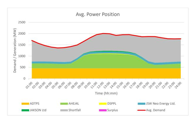
From the above Load Curve, it can be seen that there is power Shortfall in the range of  $\sim 500$  to 1100 MW and power requirement is required to be met from Short Term Open Market. Hence the procurement of 50 MW Solar will offset the short-term power requirement to that extent.
